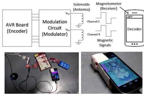
Figure 1. System architecture (top); and prototype (bottom).
