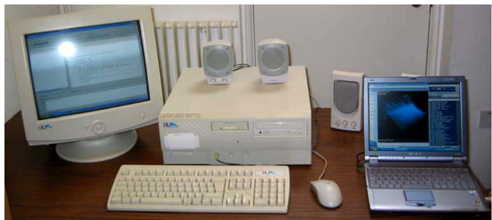
Fig. 6 The evaluators’ table with a desktop PC providing the speech output responses to the participants’ gestures and a notebook PC used to play instructions and music
