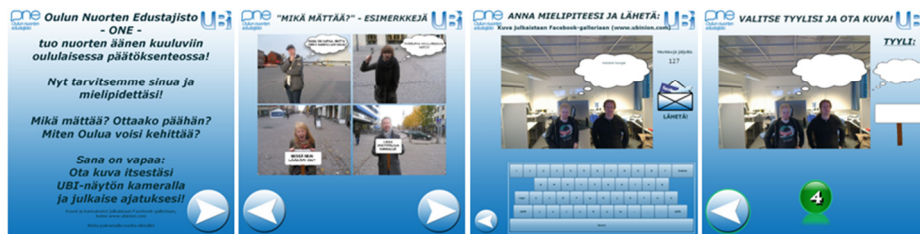
Fig 2. Ubinion’s user interface on public displays. From left: initial instruction screen, example opinions and feedback, webcam image and choice between “speech bubble” or “protest sign” as the augmenting element, and a screen with virtual keyboard to enter text in the chosen graphical element and a submit button.
