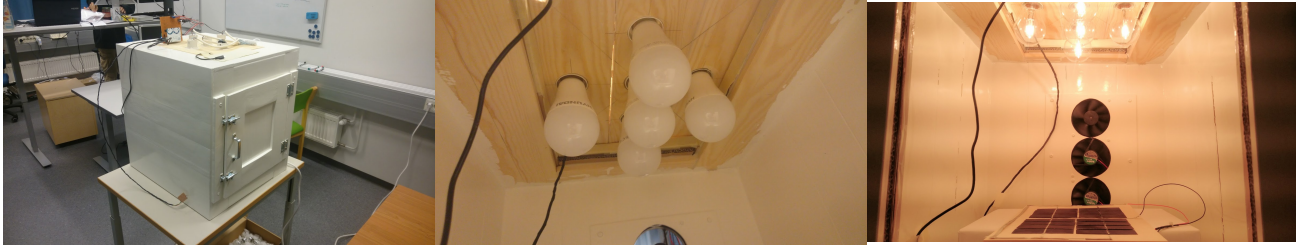
Figure 1. Our controlled environment: external light isolation, at room temperature ( \approx 21^\circ\text{C} ) and adjustable light conditions.
