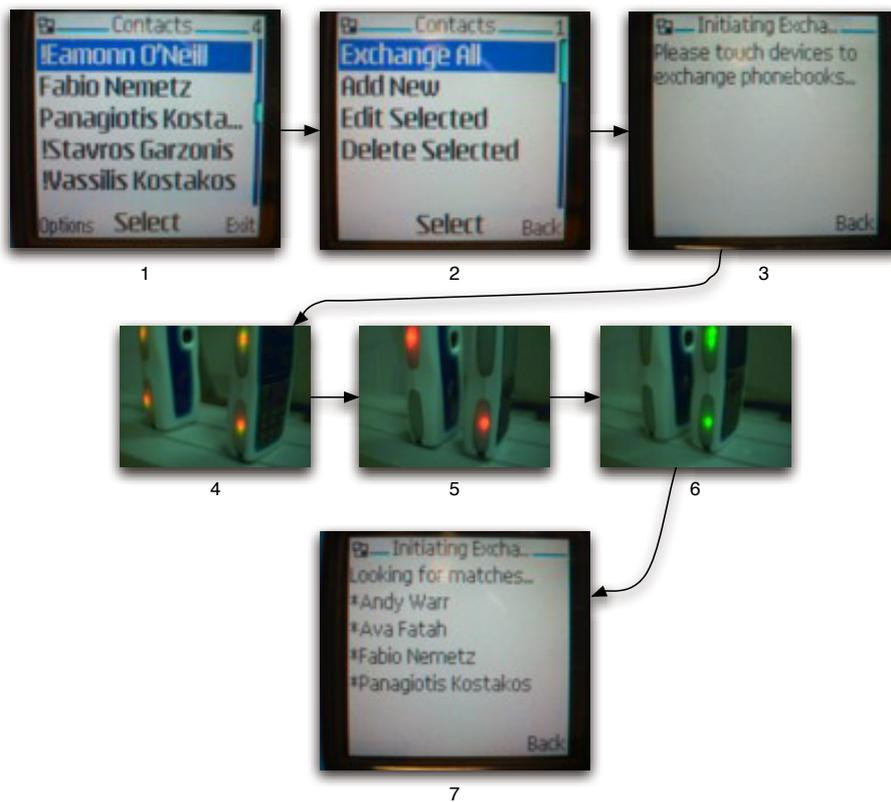
**Fig. 4.** Using NFC, both users need to activate the exchange mechanism (photos 1 to 3). The users place the phones next to each other, and wait for the exchange to take place (photos 4 to 6). The phones then display the common entries (photo 7).
