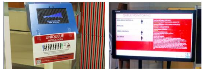
Figure 1. A kiosk that collect crowd estimations (left), and a public display displaying real-time predictions (right).
