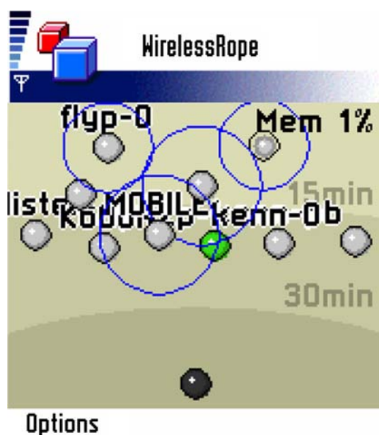
Fig. 1 A screenshot of the Wireless Rope J2ME software. The black circle represents the owner, while devices in the environment are classified as familiar ( green ) or strangers ( grey ). Devices move closer to the black circle as they spend more time within range
