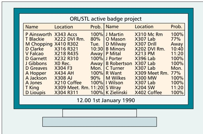
Figure 2. The Olivetti Active Badge displayed the locations of people in the laboratory and was used as an aid for a telephone receptionist to forward calls from the main switchboard [2].
