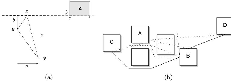
**Fig. 2.** (a) Computing the closest point  $y \in A$  to the segment  $(u, v)$ . (b) Example recomputation of connectors after deleting object A. Connectors are shown as solid lines and lower-bound connector paths through A are shown as dotted lines. The re-exploration to try and find a better path from B to C is shown as dashed lines.
