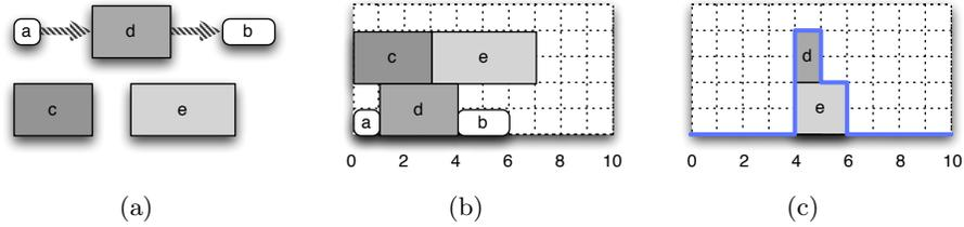
**Fig. 1.** (a) A small cumulative resource problem, with 5 tasks to place in the 5x10 box, with task **a** before **d** before **b**, (b) a possible schedule, and (c) a profile under some further conditions.
