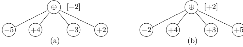
Fig. 3. XOR score (a) where the node is false and (b) where it is true
