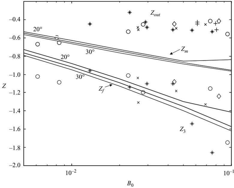
FIGURE 8. Comparison between the observed values  $Z_3$  and  $Z_m$  for all plume-like flows with the corresponding theoretical values  $Z_f$  and  $Z_{out}$ , computed for smooth slopes with slope angles of  $20^\circ$  to  $30^\circ$ . The symbols here denote: +,  $12^\circ$  slope; \*,  $20^\circ$  smooth slope; ◇,  $20^\circ$  doormat slope; ×,  $25^\circ$  slope; ○,  $30^\circ$  slope.
