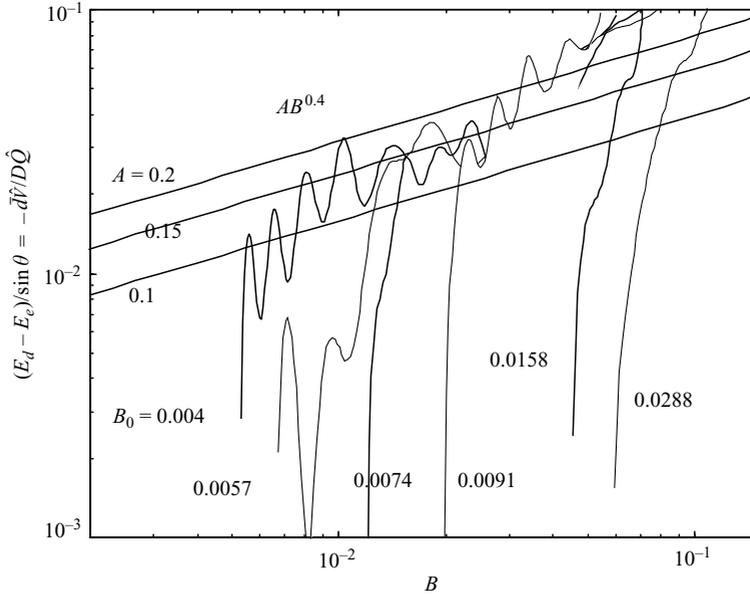
FIGURE 9. The function  $(E_d - E_e)/\sin \theta = -d\hat{V}/D\hat{Q}$ , evaluated from (5.1) in the form (5.5), plotted as a function of  $B$ , for the  $20^\circ$  doormat runs on the gravity-current side of the divide of table 2. The empirically determined form  $AB^{0.4}$  from Baines (2001) is also plotted, for  $A$  values of 0.1, 0.15 and 0.2.
