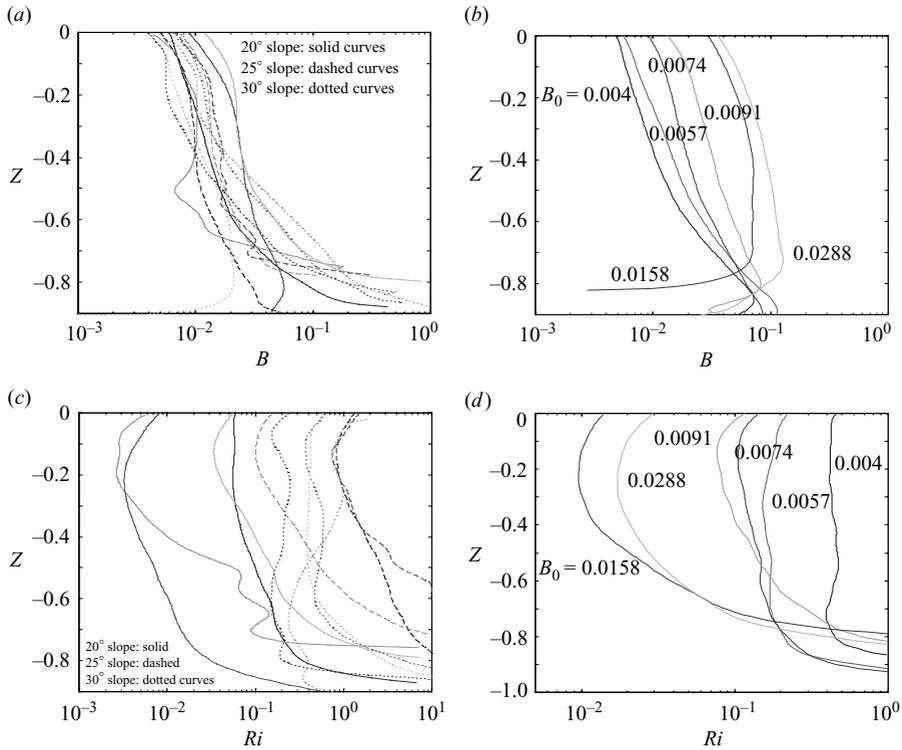
FIGURE 6. (a) Profiles of  $B(Z)$  for runs on the gravity-current side of the divide of table 2, for flow over smooth surfaces with slope angles of  $20^\circ$ ,  $25^\circ$  and  $30^\circ$ . (b) As for (a), but for doormat surface of  $20^\circ$ . (c) As for (a) but for Richardson number profiles  $Ri(Z)$ . (d) As for (b), but for Richardson number profiles  $Ri(Z)$ .
