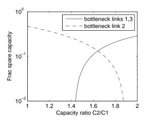
Fig. 4. Example 2: The equilibrium proportion of unused capacity on the non-bottleneck link(s) as the ratio of capacities varies, for  $C_1 = 8333 \, \text{pk/s}$ ,  $d_1 = 3 \text{ ms}, d_2 = 100 \text{ ms}$  and B = 1000 packets. For ratios between about 1.45 and 1.9, two equilibria exist: one with link 2 as a bottleneck and one with links 1 and 3 as bottlenecks.
