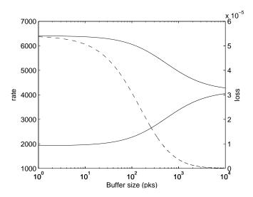
Fig. 2. Example 1. Solid lines: Rates of two fbws with different propagation delays sharing a bottleneck, as a function of buffer size. Dashed line: Corresponding packet loss probability.
