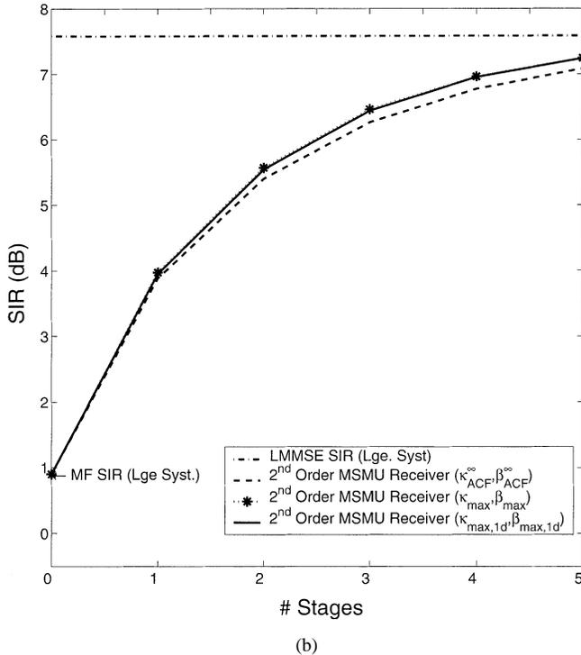
Fig. 5. Comparison of Large system SIR versus Stages, for 1-D and 2-D numerical optimization (SNR = 12 dB and  $m = 5$ ). (a)  $\alpha = 0.25$ . (b)  $\alpha = 0.75$ .
