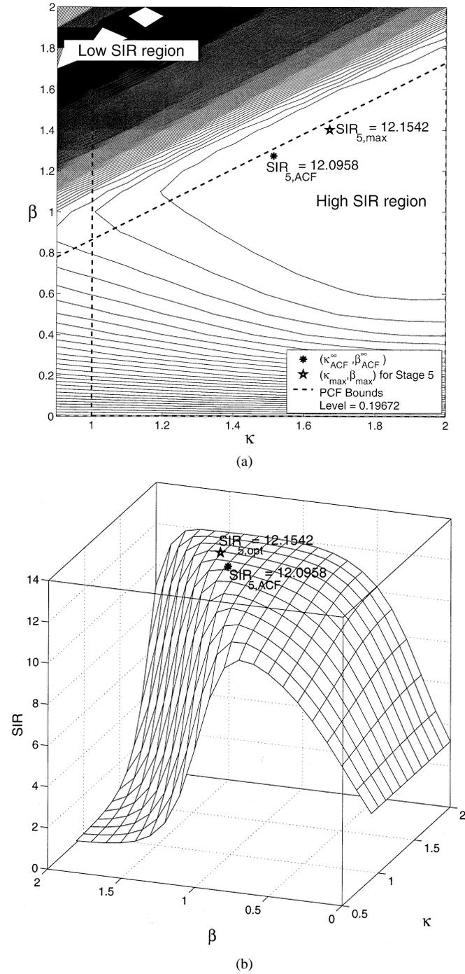
Fig. 2. Large system SIR as  $\kappa$  and  $\beta$  varies ( $\alpha = 0.25$  and SNR = 12 dB). (a) SIR contours of  $\kappa$  versus  $\beta$ .
