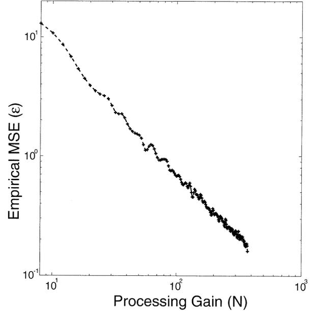
Fig. 1. Empirical mean-squared error versus  $N$  ( $m = 4$ ,  $\alpha = 0.75$ ,  $\text{SNR} = 12$  dB).
