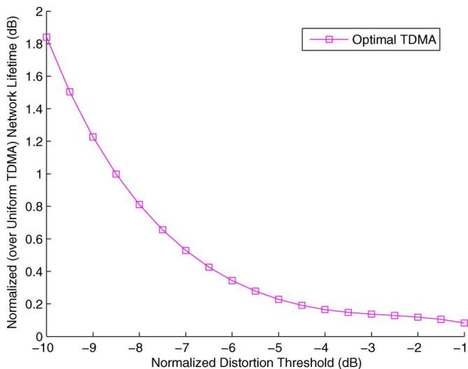
Fig. 8. Advantage of optimal TDMA over uniform TDMA.
