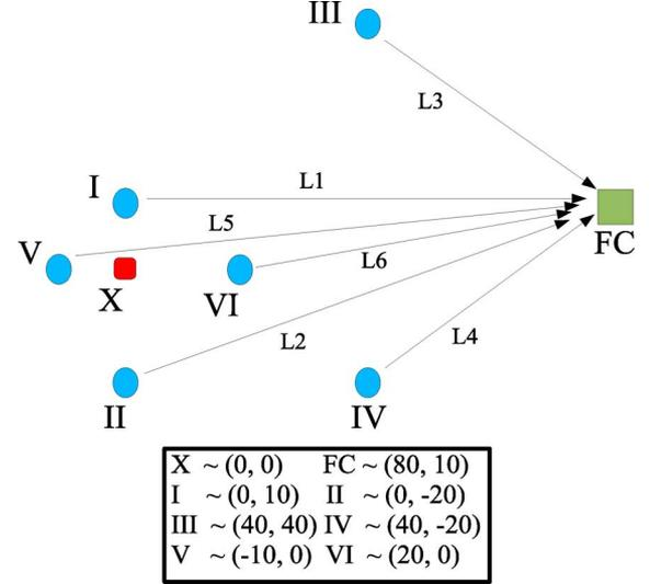
Fig. 4. Wireless detection system with six sensors (Unit: meters).
