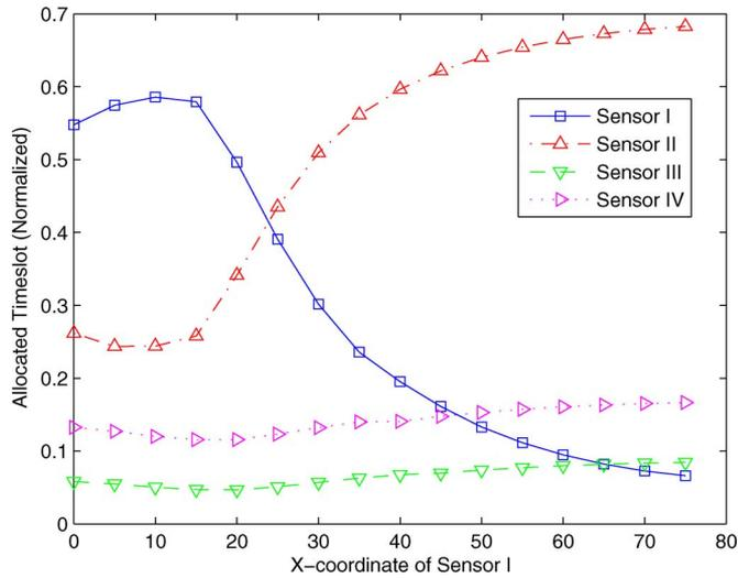
Fig. 12. Normalized sensor transmission timeslots for the (four-sensor) TDMA-based wireless sensor network with mobile sensor 1.
