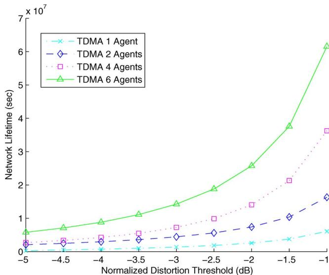
Fig. 9. Lifetime for the TDMA-based wireless sensor network.
