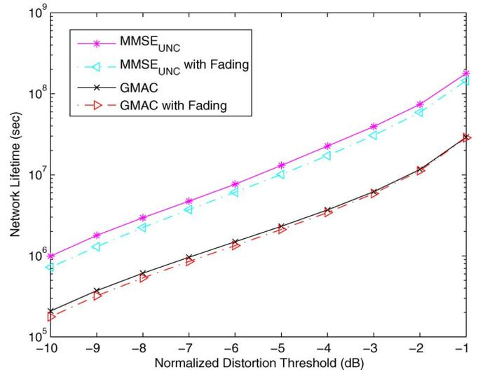
Fig. 13. Lifetime performance in Rayleigh fading – idealized GMAC and uncoded amplify and forward (MMSE<sub>UNC</sub>).
