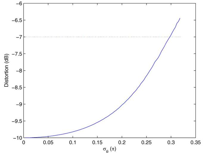
Fig. 6. MMSE distortion with phase error for the uncoded amplify and forward scheme.
