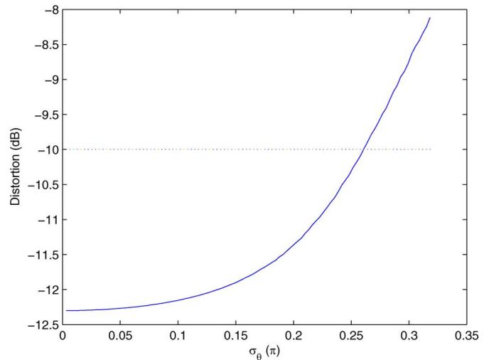
Fig. 7. MMSE Distortion with phase error for the uncoded amplify and forward scheme.
