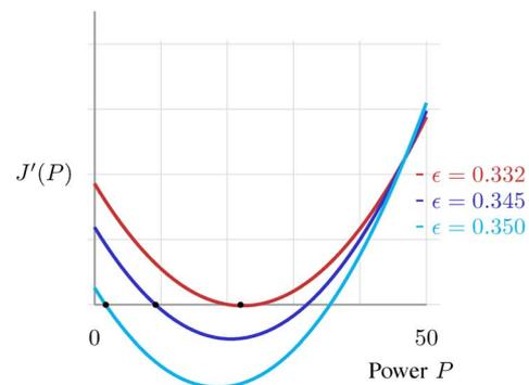
Fig. 5. Existence of local maxima when  $k = 2$  users are at  $P_{\max} = 50$ , and  $l = 1$  user is at  $P$ .
