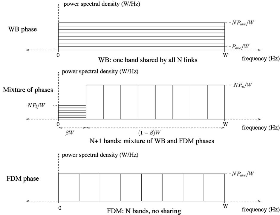
Fig. 2. Two phases and their mixture for the symmetric network of  $N$  links.
