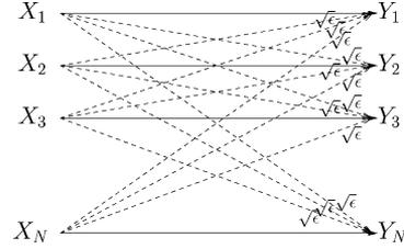
Fig. 1. Symmetric network of interfering links, where  $Y_i(t) = X_i(t) + \sum_{j \neq i} \sqrt{\epsilon} X_j(t) + Z_i(t)$ .
