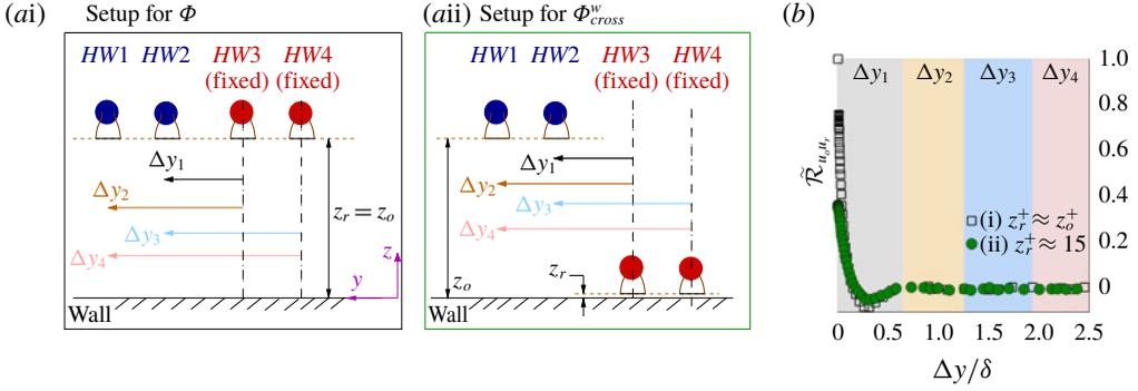
FIGURE 1. (a) Schematic of the experimental set-up in HRNBLWT showing relative positioning and movement of the four hot-wire probes ( $HW1$ – $HW4$ ) for reconstructing the 2-D correlation corresponding to (i)  $\Phi$  and (ii)  $\Phi_{cross}^w$ . Mean flow direction is along  $x$ . (b) Correlation coefficients ( $\tilde{\mathcal{R}}_{u_o u_r}$ ) as a function of spanwise separation  $\Delta y/\delta$ , computed for  $z_o^+ \approx 2.6\sqrt{Re_\tau}$  and  $\Delta x = 0$ .
