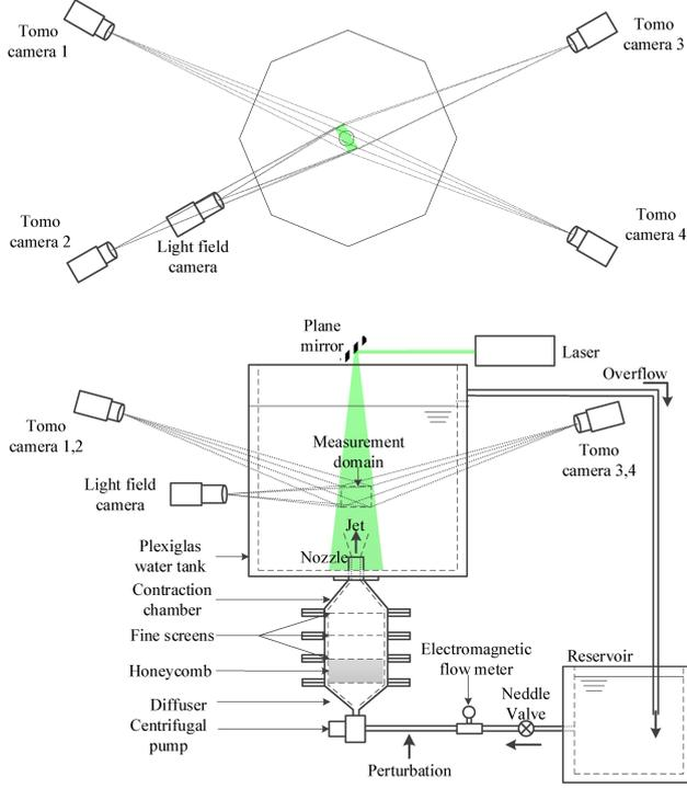
Figure 3: Typical multi-camera setup for TPIV compared to the much simpler 1 plenoptic camera LFPIV setup to measure the 3C-3D velocity field of a turbulent jet [22].
