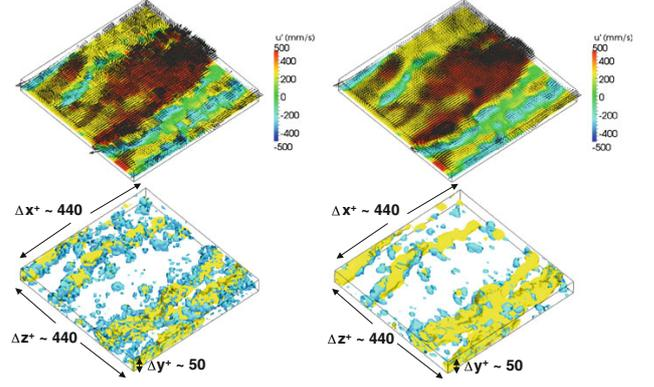
Figure 4: Instantaneous fluctuating velocity fields produced by TPIV at  $Re_{\theta} = 7,800$ . (Left) raw unfiltered velocity field and contours. (Right)  $3 \times 3 \times 3$  Gaussian filtered velocity fields and contours. Mean velocity has been removed. Vectors are shown for a single plane at  $y^+ = 27$ . *Yellow* iso-contours represent regions of low-speed velocity, *blue* iso-contours represent vortices as identified by the discriminant [32].
