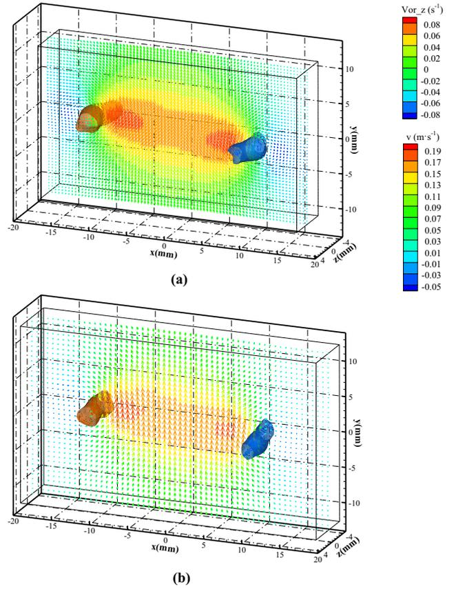
Figure 6: Phase-averaged jet flow field measured by: (a) LF-PIV and (b) Tomo-PIV of a round jet with diameter  $D = 20$  mm and  $Re_D = 2,000$  [22].
