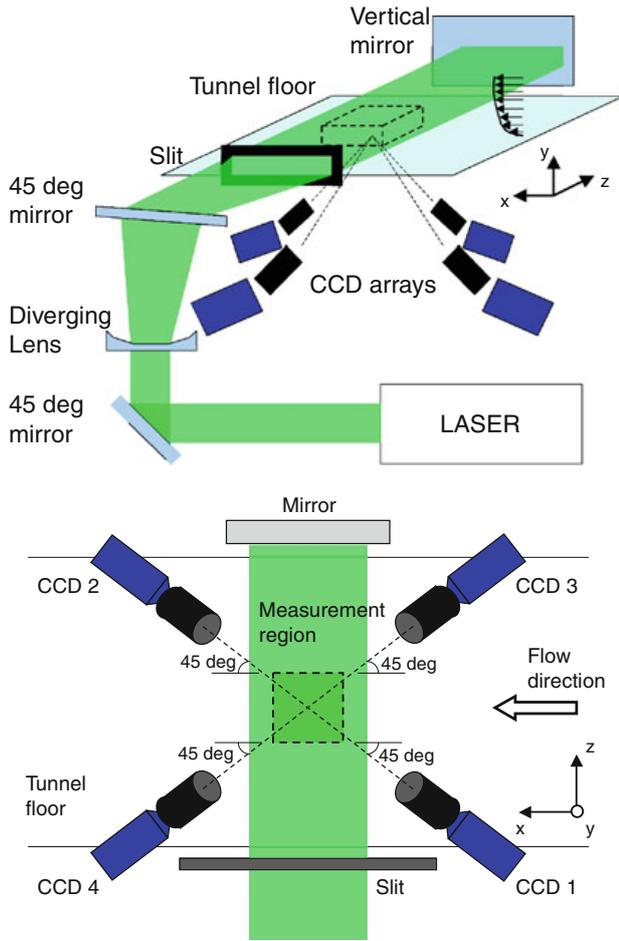
Figure 1: Typical multi-camera setup for TPIV to measure the 3C-3D velocity field of a turbulent boundary layer [17].
