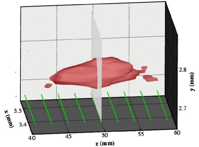
Figure 9: Digital hologram reconstruction of a 90  $\mu\text{m}$  diameter particle recorded using in-line digital holography. The central plane at  $z = 49.7$  mm is shown as a grey sheet and the green lines correspond to the locations of the other reconstruction planes [8].
