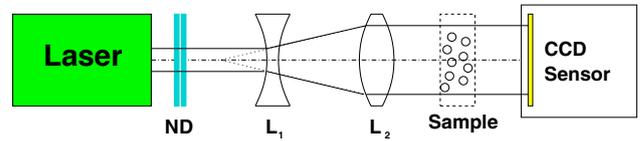
Figure 7: Typical experimental arrangement for in-line digital hologram recording (plan view), ND = neutral density filter,  $L_1$  = diverging spherical lens,  $L_2$  = converging lens.
