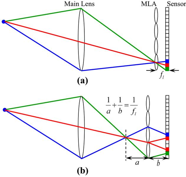
Figure 5: Schematics of light-field imaging techniques based on: (a) light- field camera and (b) focused light-field camera.
