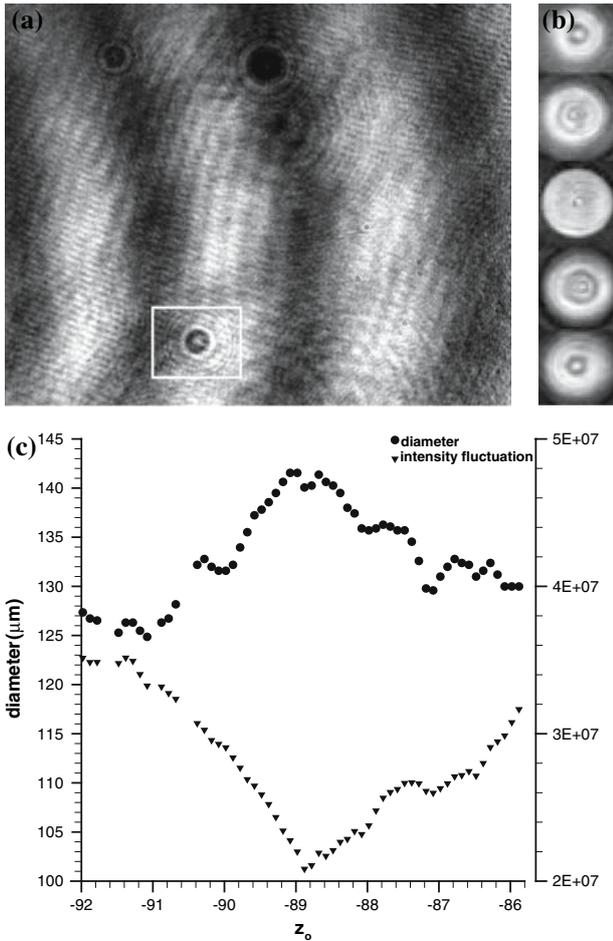
Figure 8: (a) Digital in-line hologram, (b) reconstructed particle for  $z_0$  ranging from  $-85$  to  $-93$  mm, (c) particle diameter and standard deviation of the reconstructed image intensity as a function of  $z_0$ .
