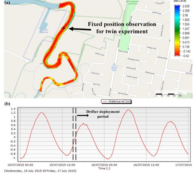
Figure 2: a: 5 m resolution bathymetry interpolation of the Erapah Creek (\* represents the location of the fixed position observation for twin experiment) and b: time series of the water level and drifter deployment period.
