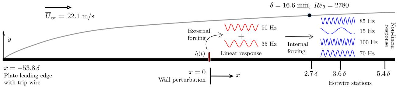
Figure 3: Schematic of dynamic roughness experiments, from Duvvuri and McKeon [3]. A spanwise element is oscillated at one or two frequencies to excite linear and nonlinear responses in a turbulent boundary layer, which are reconstructed by phase-locking downstream measurements to the phase of the dynamic roughness actuation.
