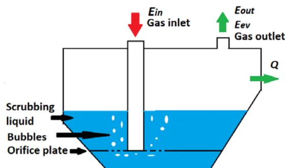
Figure 1. Exhaust wet scrubber schematic diagram.
