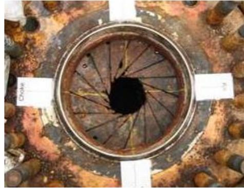
Figure 1. Photo of the upper annular preventer recovered from the Macondo BOP stack after it was sealed [1].
