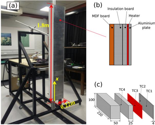
Figure 1 Experiment setup and constitutive unit: (a) Photo of experiment setup, showing the flat plate and mounting frame assembly. Yellow arrow denotes the location coordinate starting from the leading edge; (b) Side-view of one representative heating unit, showing components; (c) Exploded view of heating unit, showing thermocouple (TC) locations as well as dimensions of components. Note that dimensions are in millimetres.
