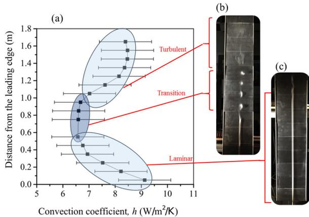
Figure 7. (a) Variation of convection coefficient along a vertical plate for 818 W/m<sup>2</sup> uniform flux experiment, without sidewalls, (b)-(c) Photos of smoke visualisation during experiment, qualitatively showing turbulent and laminar flow regimes, respectively.
