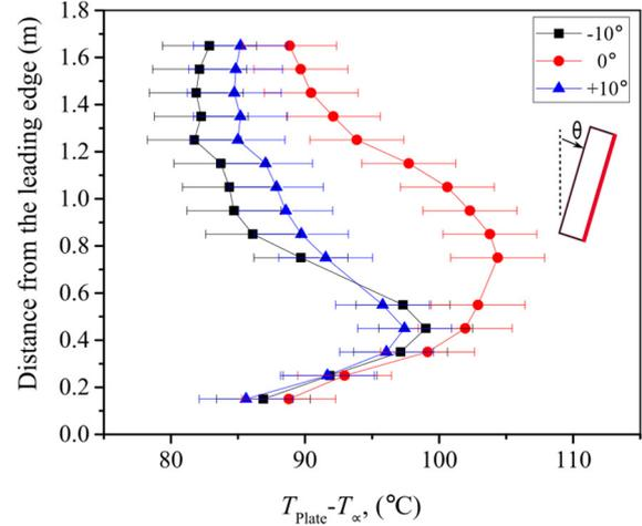
Figure 5 Temperature distribution along the length of the heated plate, with sidewalls, as a function of inclination angle. Total input flux is kept constant and uniform at  $818 \text{ W/m}^2$ . Inset shows the positive angle definition, with the heated plate shown in red.
