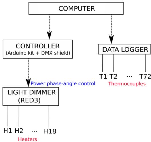
Figure 2 Schematic of the power control system used for the experiments
