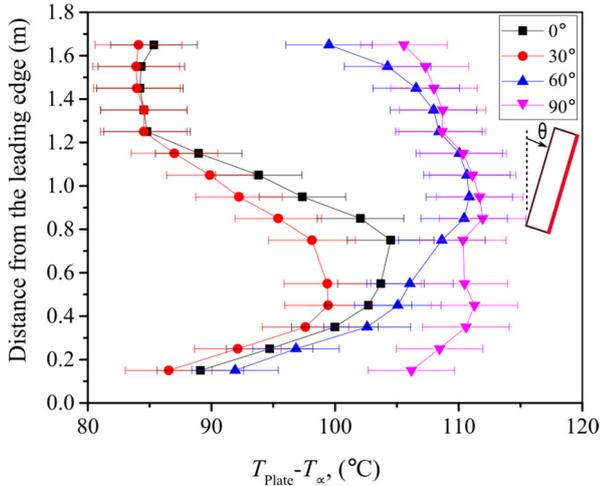
Figure 4 Temperature distribution along the length of the heated plate, without sidewalls, as a function of inclination angle. Total imposed flux is kept constant and uniform at  $818 \text{ W/m}^2$ . Inset shows the positive angle definition, with the heated plate shown in red.
