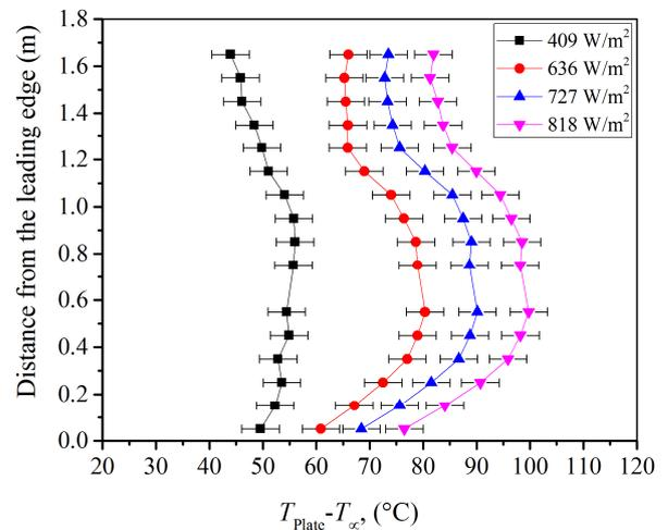
Figure 3. Temperature distribution along the length of the vertical heated plate without sidewalls, for different values of imposed uniform flux.
