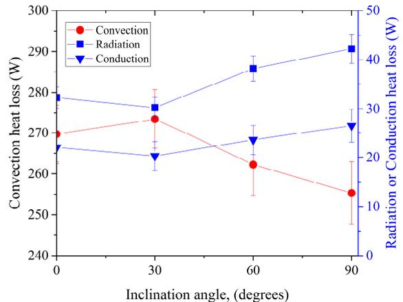
Figure 6. Heat loss from the flat plate as a function of angle, subject to uniform flux boundary condition, without sidewalls.
