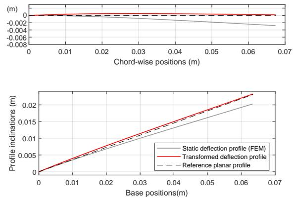
Figure 4: Convex profile obtained through an anticlockwise angular transformation of the baseline profile, plotted with respect to the horizontal (top) and the inclined planar profile (bottom).
