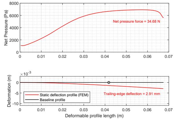
Figure 3: Pressure distribution and static deformation profile.
