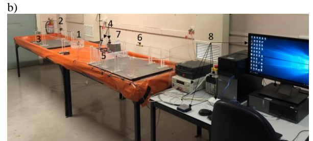
Figure 2. a) Schematic of the test setup and b) Experimental test setup: (1) centrifugal pump; (2) flow sensor; (3) settling chamber; (4) pressure sensor; (5) 3D-printed test section; (6) valve; (7) water reservoir; (8) computer, power supply and DAQ card.
