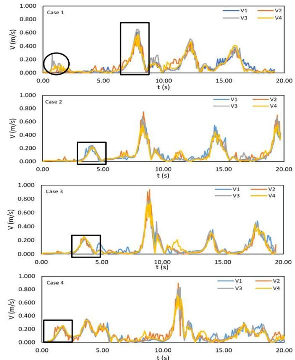
Figure 5 Velocity profiles of CLPHP.
