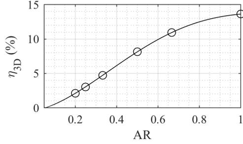
Figure 3: Three-dimensionality parameter as a function of the aspect ratio.
