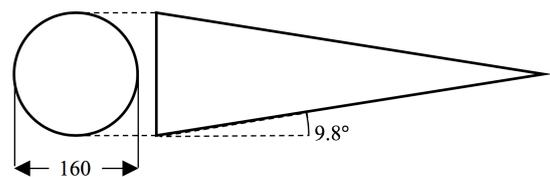
Figure 1: Nominal core-flow (dimensions in millimetres).
