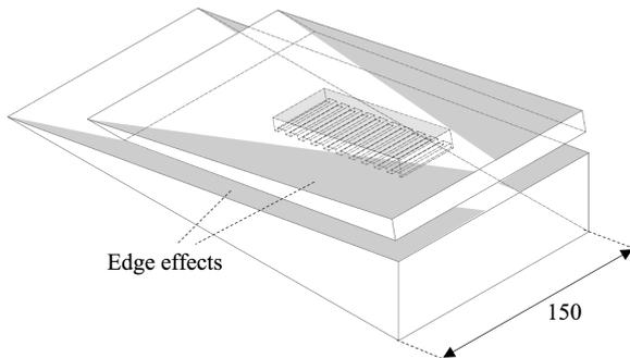
Figure 9: Isometric drawing of the wind-tunnel model with detail of the edge-effects extent on both plate and ramp. (dimensions in millimetres).
