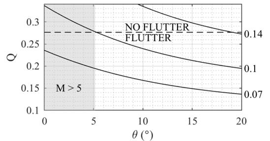
Figure 5: Flutter boundaries for  $AR = 0.4$  and  $\Delta p \sim 0$ . Present values of  $Q$  are plotted for three different values of thickness (namely 0.07, 0.1 and 0.14 mm).
