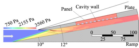
Figure 7: Side view of the wind tunnel model and laminar pressure solution (dimensions in millimetres).
