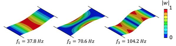
Figure 4: First three (computed) modes for a plate with a length of 100 mm, a thickness of 0.07 mm and an aspect ratio of 0.4.
