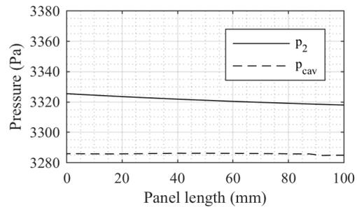
Figure 8: Pressure acting on the windward and cavity side of the plate from laminar CFD.
