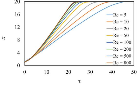
Figure 3: Passage of the intrusion front for a series of  $Re$  with  $Fr = 1$  and  $Pr = 7$ , where  $x = X/X_0$  and  $\tau = (tW_0)/X_0$  are the dimensionless  $x$ -location and time.
