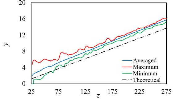
Figure 5: Passage of the thermally stratified surface for the fountain with  $Fr = 1.0$ ,  $Re = 200$  and  $Pr = 7$ .
