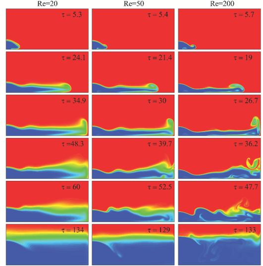
Figure 2: Temperature contours for the fountains of  $Fr = 1$  and  $Pr = 7$ . The left, middle and right columns are for  $Re = 20$ ,  $Re = 50$  and  $Re = 200$  at six specific times, respectively.
