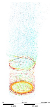
Figure 2. Schematic diagram of swirling flows caused by rotating the tower wall.
