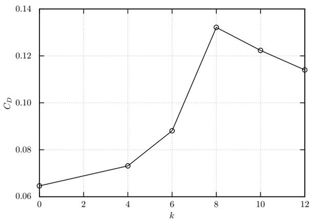
Figure 8: Variation of the drag coefficient  $C_D$  with the roughness wave number  $k$ .
