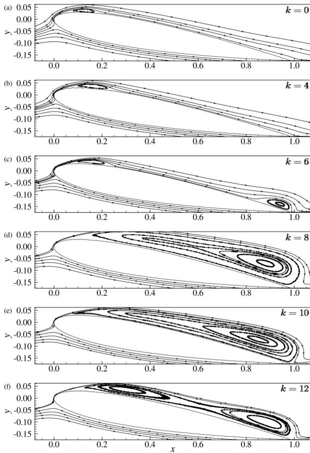
Figure 5: Streamlines of the time and spanwise-averaged flow field for different roughness wave number.
