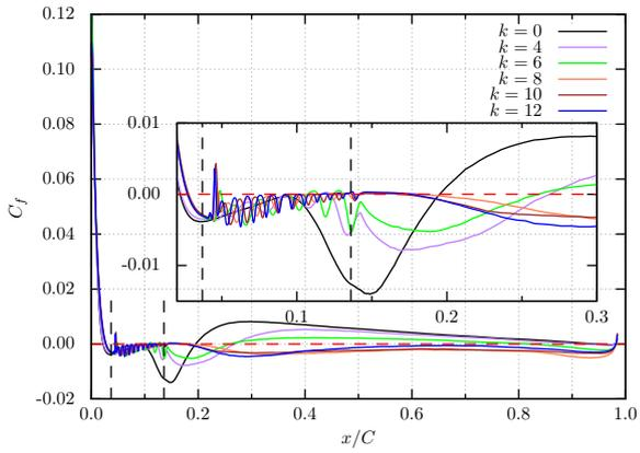
Figure 4: Distribution of the time- and spanwise-averaged friction coefficient  $C_f$  on the suction side. The black dash lines denotes the boundary of the roughened region, and the red dashed lines denotes  $C_f = 0$ .
