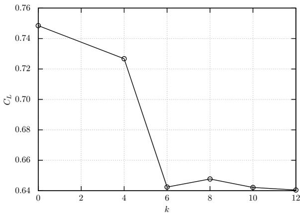
Figure 7: Variation of the lift coefficient  $C_L$  with the roughness wave number  $k$ .
