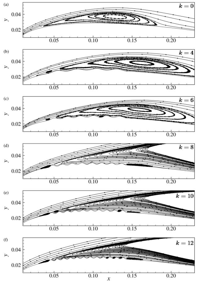
Figure 6: Streamlines of the time and spanwise-averaged flow field near the roughened region for different roughness wave number.
