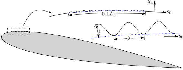
Figure 1: Sketch of the NACA0012 airfoil with artificial wavy roughness elements.  $s_0$  and  $y_n$  denotes the local coordinate direction parallel and normal to the smooth airfoil surface ( $k = 0$ ), respectively.
