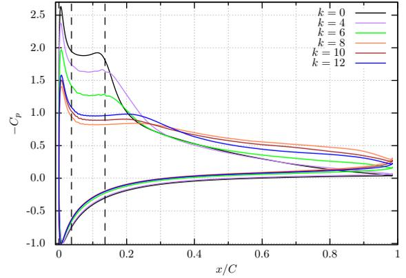
Figure 3: Distribution of the time- and spanwise-averaged pressure coefficient  $C_p$  around the airfoil. The black dash lines denotes the boundary of the roughened region.
