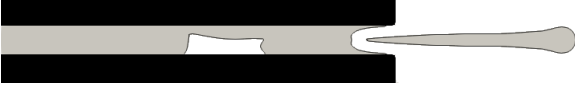
Figure 2: Elevation in the plane of left-right symmetry showing ink (grey) and airy 'bubble' (white) after 30\ \mu\text{s} , simulated with interFoam ; cf. [3, figure 3]
