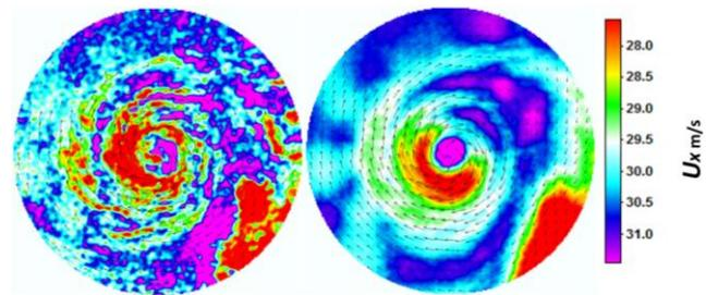
Figure 2. Left: an instantaneous velocity field of the fin-tip vortex at 65% of the model length. Right: reconstruction of the same instantaneous velocity field based on the first three modes from the POD analysis. The contour levels represent the out-of-plane streamwise velocity ( $U_x$ ).
