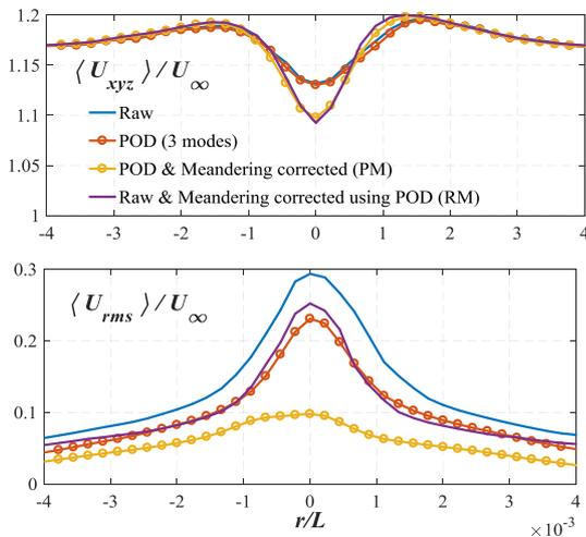
Figure 10. The normalized resultant velocity and fluctuation of Raw, POD approximated, POD & Meandering corrected and Raw & Meandering corrected using POD results at  $65.0\%L$ .
