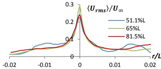
Figure 7. The turbulence intensity of the selected fin-tip vortex at three measurement planes.
