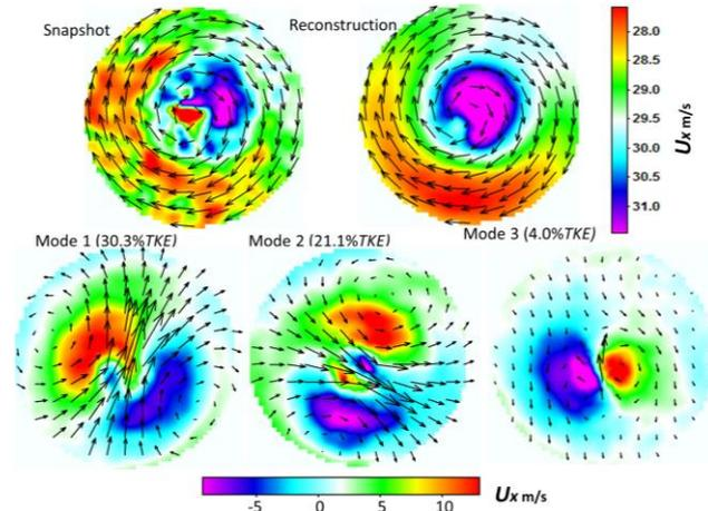
Figure 5. Top: an instantaneous velocity field of the vortex core and the reconstruction of the flow field based on the first three modes. Bottom: first three POD modes with their eigenvalues/energy level.
