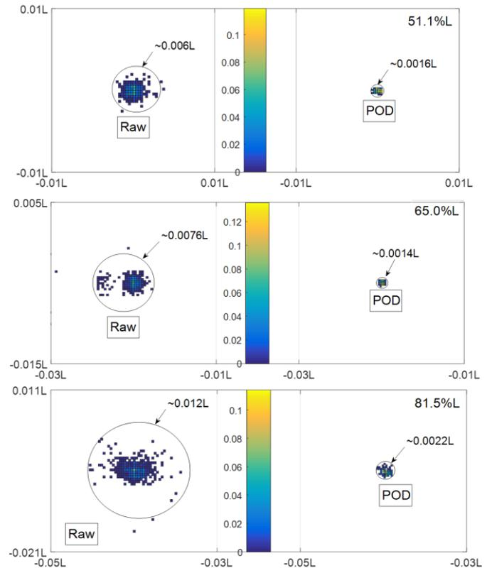
Figure 9. Probability density function (PDF) of the instantaneous vortex centre of the raw and POD-corrected velocity vectors identified by the minimum vorticity at three axial locations along the model.
