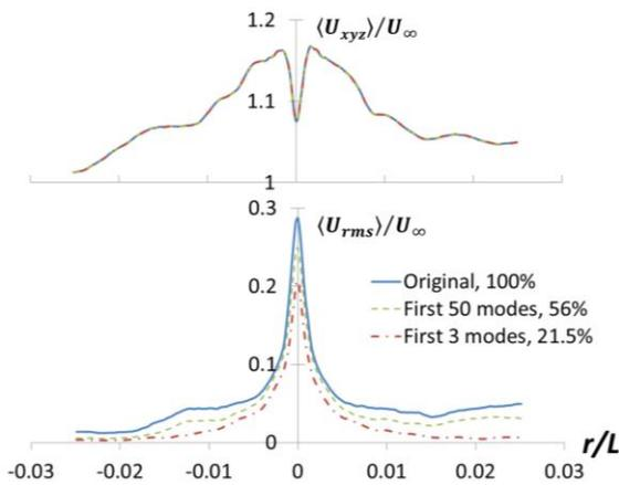
Figure 8. The normalized resultant velocity and the turbulence intensity of the original raw data, the POD approximation (first 50 modes, 56% of total turbulent energy) and the POD approximation (first 3 modes, 21.5% of total turbulent energy) at 65%L.
