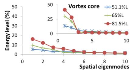
Figure 6. Eigenvalue distribution of the 1000 snapshots of the fin-tip vortex (main figure) and the vortex core (top right) at three measurement planes along the model.
