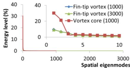
Figure 4. Contributions from the POD eigenmodes to the total energy for different cases with a particular focus on the first ten modes (1000 snapshots of fin-tip vortex, 3000 snapshots of fin-tip vortex and 1000 snapshots of the vortex core).
