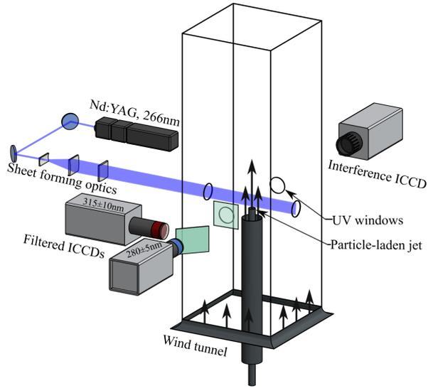
Figure 2: Experimental setup for two-colour LIF thermometry of particle-laden jets
