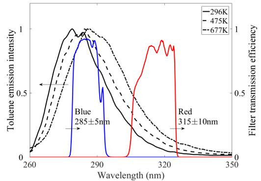
Figure 1: Normalised toluene fluorescent emission spectrum at different temperatures (adapted from [3]) and optical filter transmission efficiencies of the fluorescence cameras
