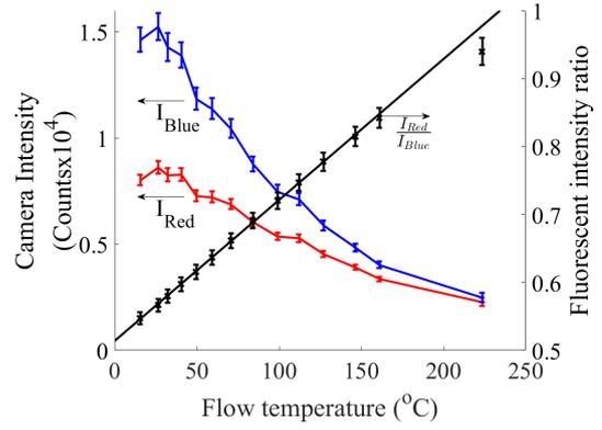
Figure 3: Calibration data for intensity ratio of a toluene seeded heated jet. The solid line shows a curve fitted to the data. Also shown is the average camera counts for the red and blue channels. Error bars are one standard deviation either side of the mean.
