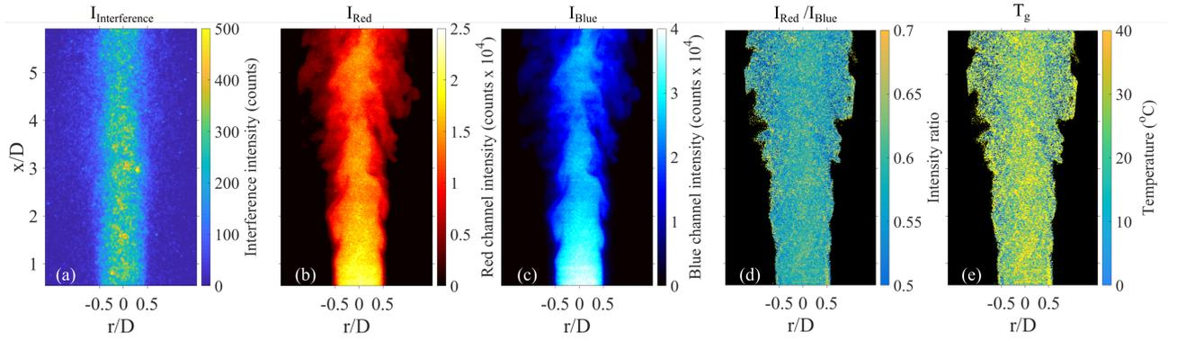
Figure 4: Images used in processing - (a) is a single-shot particle interference image, (b) and (c) are the single-shot images from the red and blue fluorescence cameras captured simultaneously with (a), (d) is the intensity ratio image, (e) is the temperature image
