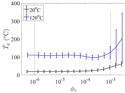
Figure 6: Effect of particle loading on mean temperature calculation. Error bars show one standard deviation either side of the mean value. The dashed vertical lines indicate the boundaries of the two-way coupling regime
