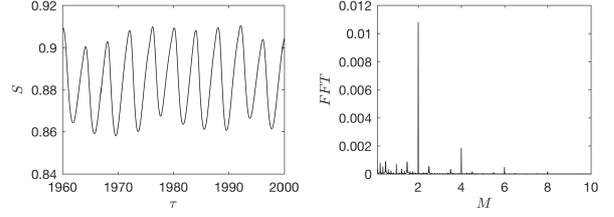
Figure 4: Stratification time series (left) and fast Fourier transform (right) for  $Ra = 1 \times 10^8$ ,  $Pr = 0.7$  and  $f = 0.125$ .
