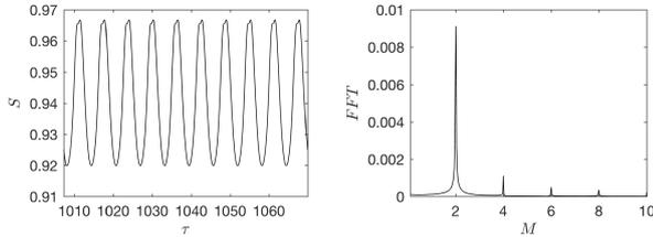
Figure 3: Stratification time series (left) and fast Fourier transform (right) for  $Ra = 1 \times 10^8$ ,  $Pr = 0.7$  and  $f = 0.08$ .
