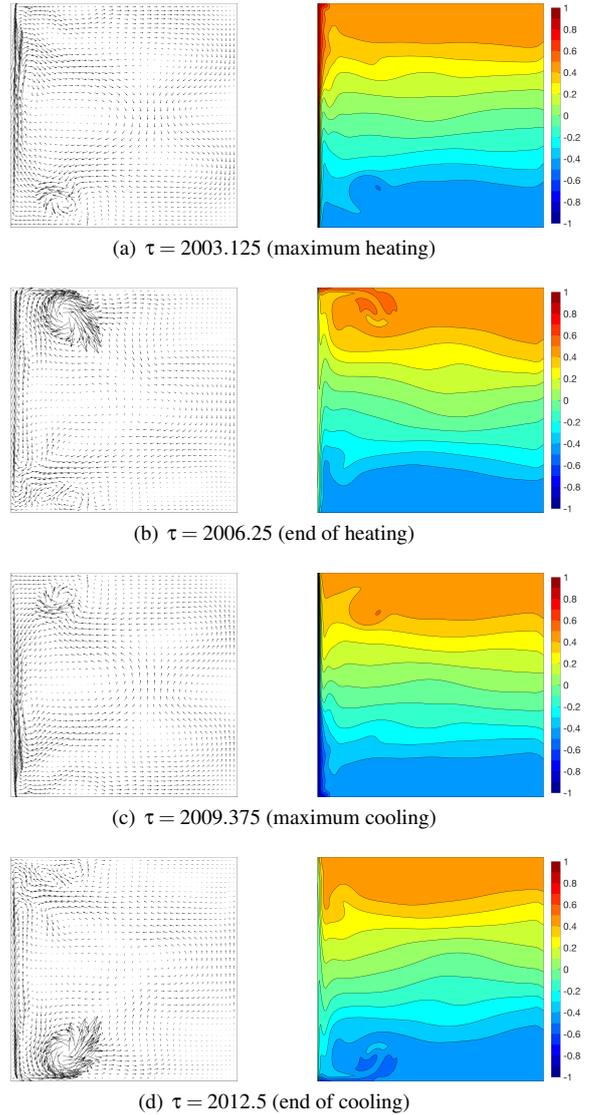
Figure 2: Velocity vectors (left) and temperature contours (right) for  $Ra = 1 \times 10^8$ ,  $Pr = 0.7$  and  $f = 0.08$ .
