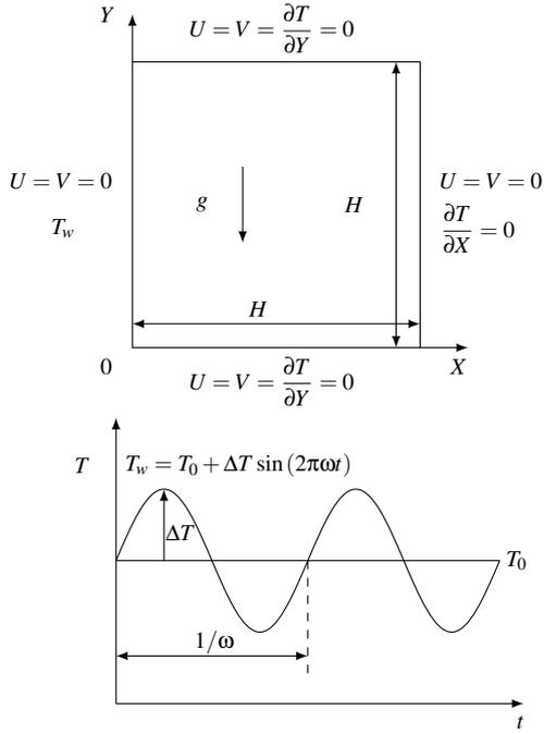
Figure 1: Flow setting and thermal forcing.
