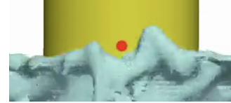
Figure 5: Screenshot of a CFD result highlighting how the averaging processing in the visual tracking algorithm can occasionally measure a D_1 value (red dot) higher than the bow wave height directly at the front of the cylinder, when the free surface in the immediate vicinity is higher.
