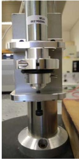
Figure 1. The extensional viscometer.
