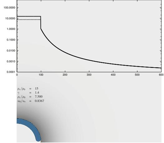
Figure 1: Meridional section through one quadrant of the flow field around a hollow spherical moon with an opening at a pole, showing the initial conditions for the computation. The greys shading is proportional to the magnitude of the fractional density gradient and illustrates the variation through the (here isothermal) atmosphere. The plot at the top shows pressure (heavy line) and density profiles.
