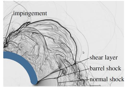
Figure 2: Example of results of computation of the flow.  $p_r/p_0 = 60$ ,  $u_0/u_{eg} = 0.837$ ,  $\gamma = 1.4$ ,  $r_*/r_0 = 0.1$ .
