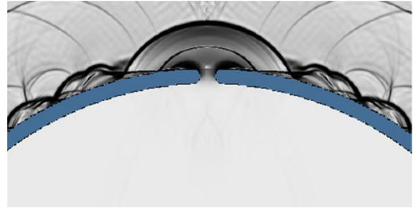
Figure 6: Image from one of the computations of the volcano Tvashtar. Note how the structure of this flow differs from cases with larger  $u_0/u_{eg}$  such as the one in figure 2. It is like a smooth dome, similar to that in the image of Tvashtar, figure 4. The shock waves visible above the dome appear stronger than they are, because the greyscaling is proportional to the fractional density gradient.
