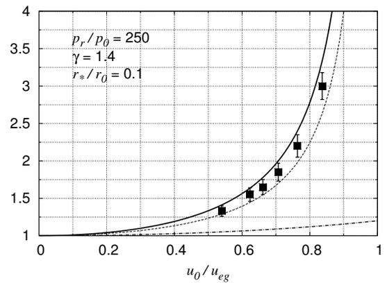
Figure 3: Plot of dimensionless steady-state jet penetration radius  $r_p/r_0$  vs.  $u_0/u_{eg}$  for  $\gamma = 1.4$ ,  $r_*/r_0 = 0.1$ .  $p_r/p_0 = 250$ . The full line shows the value given by equation (9). The dotted line indicates results with  $p_r/p_0 = 15$ . The chain-dotted line indicates the penetration radius of a solid body with the same surface speed.
