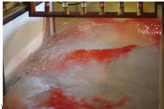
Figure 1. Compression wave propagation in an asymmetrical trapezoidal channel. (a) Un-distorted definition sketch. (b) Looking downstream for Q = 0.026 \text{ m}^3/\text{s} , Fr_1 = 1.45 . (c) Looking downstream for Q = 0.054 \text{ m}^3/\text{s} , Fr_1 = 1.4 , with dye injection.
