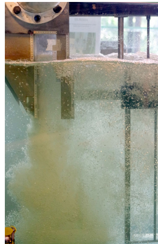
Figure 1. Air entrainment at a vertical supported jet. Flow conditions: V_1 = 4.5 m/s, d_1 = 0.0114 m, Fr_1 = 13.5 , Re_1 = 5.14 \times 10^4 .
