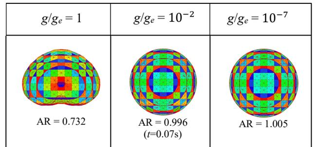
(b) 4 mm bubble,  $\Delta T_{super} = 1^\circ\text{C}$ , Simulation time = 0.134 s
