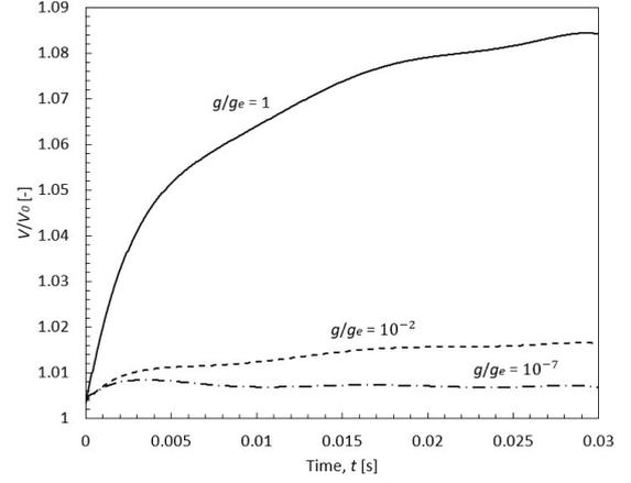
(a) For various gravity levels (2.5 mm bubble,  $\Delta T_{super} = 35^\circ\text{C}$ )
