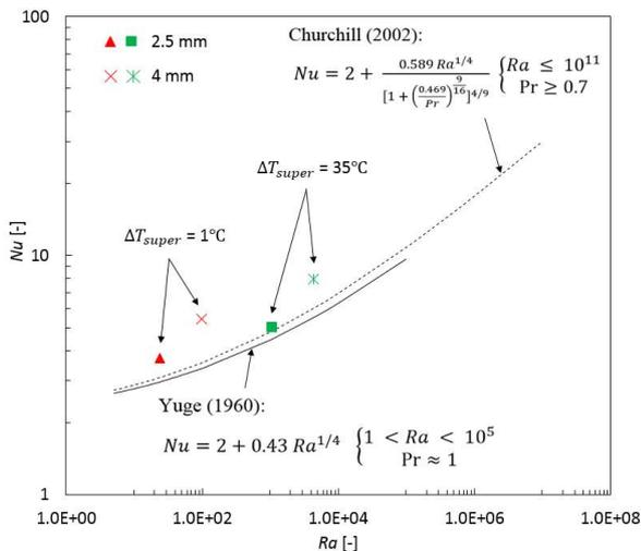
Figure 3. Natural Convection data for vapour bubble in micro-gravity environment ( $g/g_e = 10^{-2}$ )
