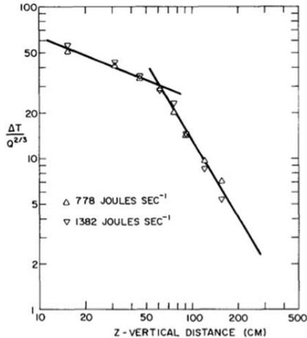
Figure 5. Scaled Temperature Excess vs Height (Mullen and Maxworthy [8])
