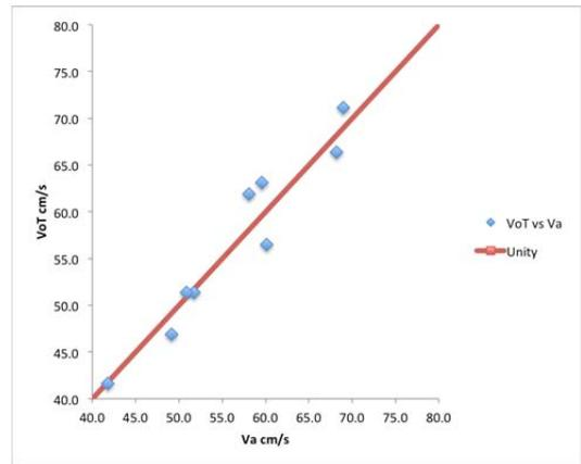
Figure 6. Tangential Velocity – modelled and measured
