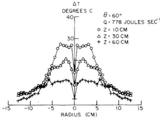
Figure 4. Scaled Temperature excess vs Radius, 60° vane angle, 778W (Mullen and Maxworthy [8])
