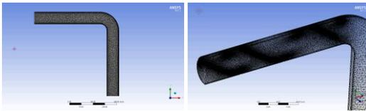
Figure 2. Mesh on 3in Plain 90° Pipe Bend (left), Mesh on 3in 90° Pipe Bend with passive flow control with swirl C (right).
