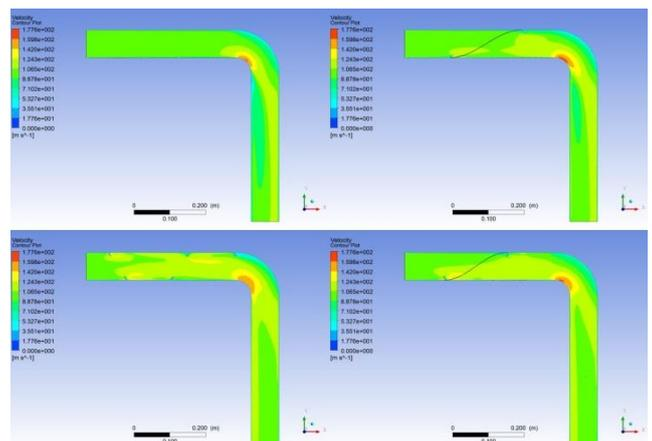
Figure 4. Velocity Contour, steady state,  $100 \text{ ms}^{-1}$  inlet flow, clockwise from top left; Base, swirl A, swirl B & swirl C.
