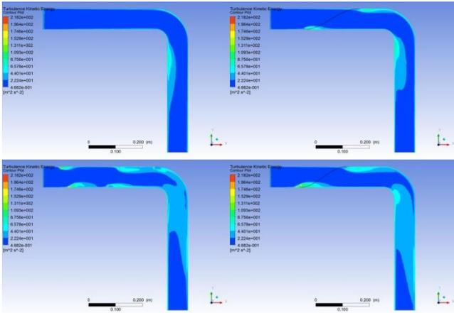
Figure 5. Turbulent Kinetic Energy Contour, steady state, 100 ms<sup>-1</sup> inlet flow, clockwise from top left; Base, swirl A, swirl B & swirl C.
