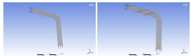
Figure 1. 3in Plain 90° Pipe Bend. R/D = 1 (left), 3in 90° Pipe Bend with passive flow control with swirl C(right).
