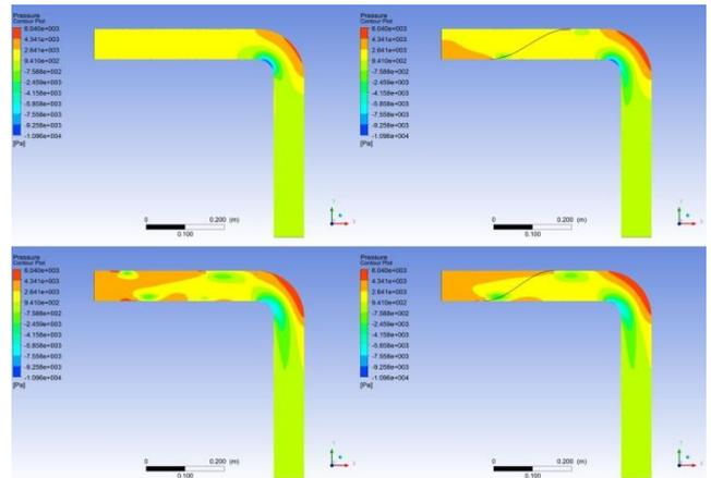
Figure 3. Pressure Contour, steady state,  $100 \text{ ms}^{-1}$  inlet flow, clockwise from top left; Base, swirl A, swirl B & swirl C.
