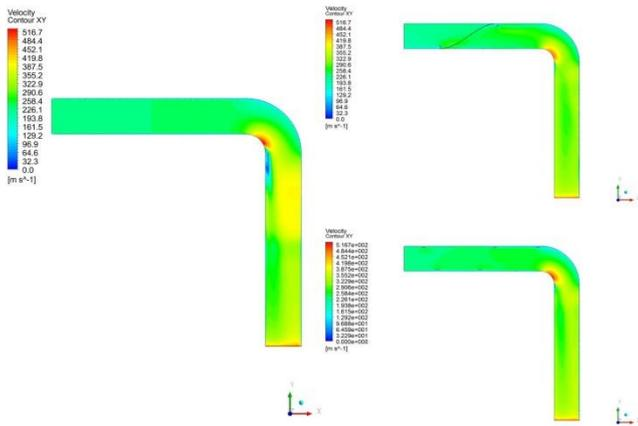
Figure 6. Velocity Contour, steady state, 100 ms<sup>-1</sup> inlet flow, clockwise from left; Base, swirl C, & swirl D.
