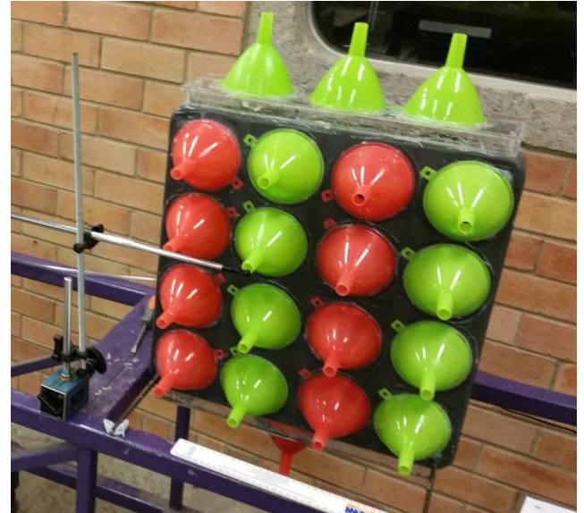
Figure 2. Green-wall module with funnels attached (16 covering the front openings, 3 on top and 1 at bottom). The hot-wire velocity probe can be seen at the black right end of the silver-colour horizontal handle; the handle itself is mounted on an aluminium vertical post seen at the left of the module.
