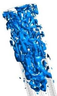
Figure 10: Isocontour of an oil volume fraction of 0.1 at 1000RPM
