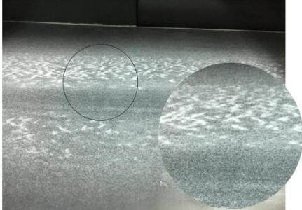
Figure 7 the pattern on the plate ( $Sn = 100$ , smooth plate)
