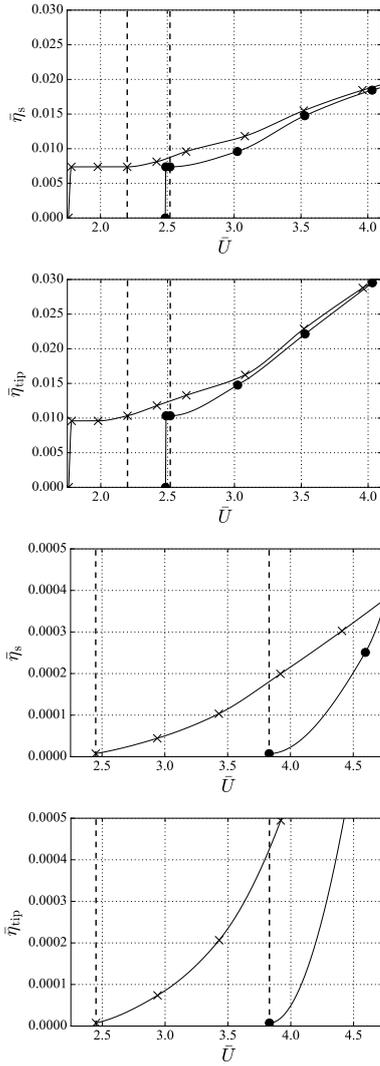
Figure 3: Maximum displacement for increasing  $\bar{U} = U_c(1 + \Delta)$  with  $\bar{L} = 1$  &  $\bar{\gamma} = 1 \times 10^4$ : Top two figures -  $\bar{\omega}_s = 1$ , Bottom two figures -  $\bar{\omega}_s = 10$ ;  $\times d^+ = 0$ ,  $\bullet d^+ = 0.1$ . The left and right vertical dashed lines denote  $U_c$  values for the linear cases without and with damping respectively. 1st and 3rd figures: mount, 2nd and 4th figures: tip.
