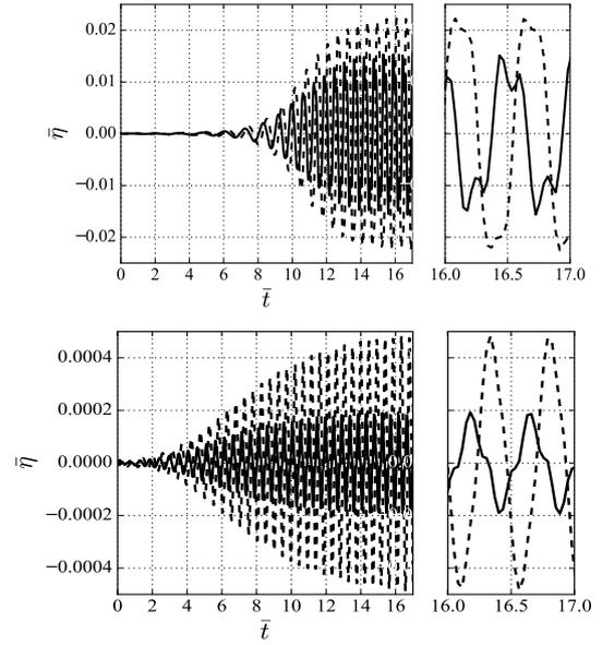
Figure 2: Displacement in time for  $\Delta = 0.6$  with  $d^+ = 0$ ,  $\bar{L} = 1$  &  $\bar{\gamma} = 1 \times 10^4$ : — Mount, - - Tip; Top -  $\bar{\omega}_s = 1$ , Bottom -  $\bar{\omega}_s = 10$ . Small windows show traces from  $\bar{\tau} = 16$  to 17.
