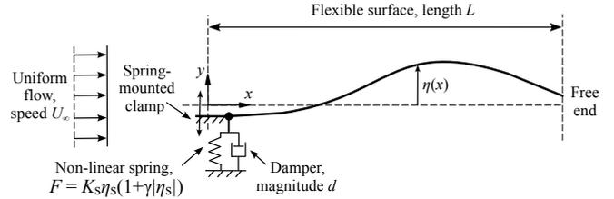
Figure 1: The fluid-structure system under consideration.
