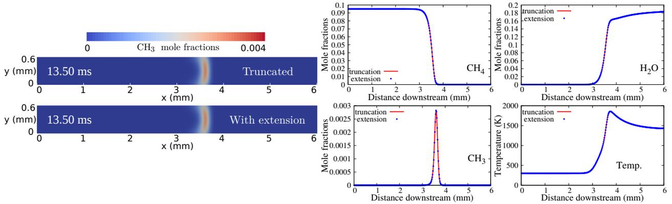
Figure 3: Contour of  $\text{CH}_3$  mole fractions (left), and profiles of species and temperature along the channel centreline (right) of the steady-state flame solutions ( $U_{in} = 0.4$  m/s), using a truncated computational domain and a domain with an extension.
