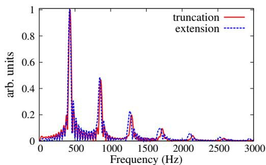
Figure 6: Fast Fourier transform of the THRR for two types of outflow boundary treatments, showing the predominant frequencies of flame oscillations.
