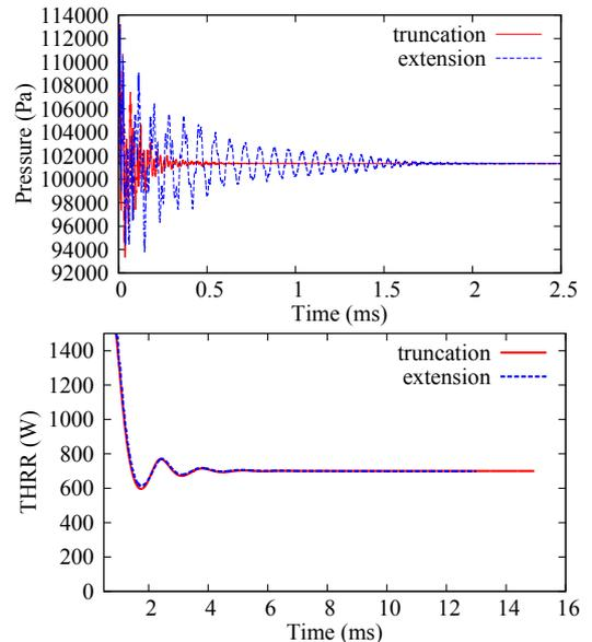
Figure 2: Pressure variations at the monitored point (located at the centre of the combustor zone) and *THRR* evolutions for two types of outflow boundary treatments, at  $U_{in} = 0.4 \text{ m/s}$ .
