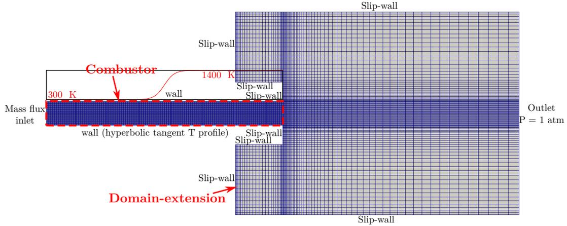
Figure 1: Computational domain showing the truncated planar combustor and the domain-extension joining the combustor outlet.
