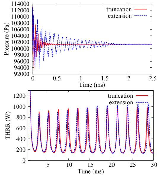
Figure 4: Pressure variations at the monitored point (located at the centre of the combustor zone) and  $THRR$  evolutions for two types of outflow boundary treatments, at  $U_{in} = 0.2$  m/s.
