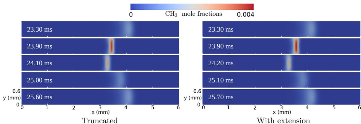
Figure 5: Temporal evolution of the oscillating flames ( $U_{in} = 0.2$  m/s) within one cycle, using a truncated computational domain and a domain with an extension.
