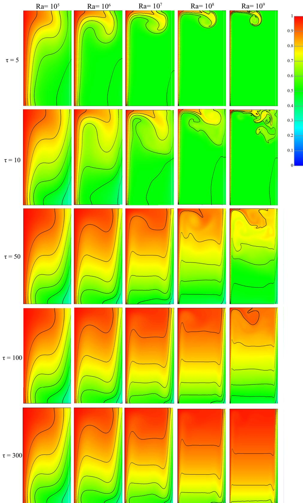
Figure 2: Temperature contours on the left enclosure at different times.
