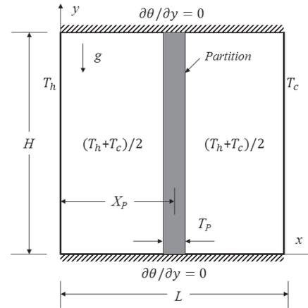
Figure 1: Schematic of the physical model, the computational domain and the boundary conditions.
