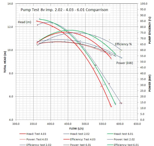
Figure 10. Pump curves for 8-vane impeller. Test numbers 2.02, 4.03 and 6.01 are explained in Table 2.
