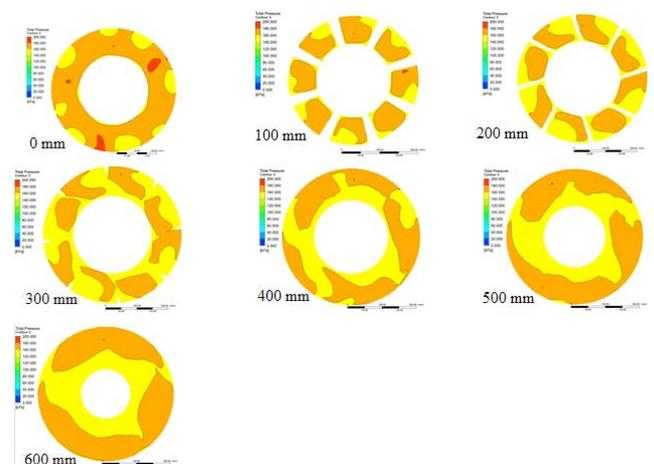
Figure 4. Total pressure on sections through the combined new-diffuser and tail-piece for five vane impeller. Dimensions 0 mm to 600 mm indicate the distance downstream from the diffuser's inlet face.
