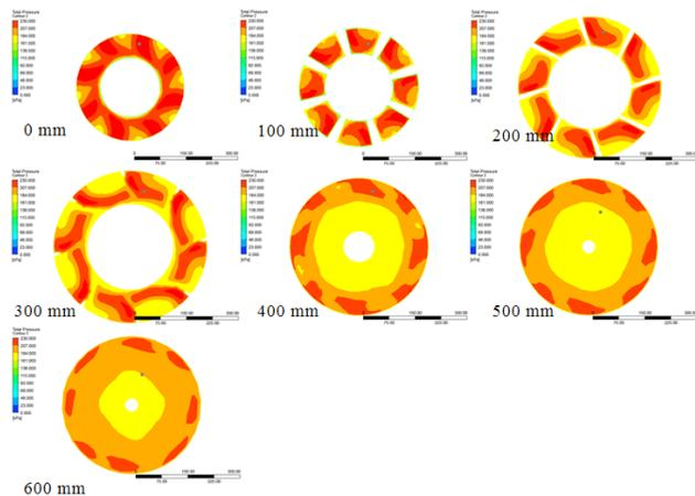
Figure 5. Total pressure on sections through the new diffuser for eight-vane impeller. Dimensions 0 mm to 600 mm indicate the distance downstream from the diffuser's inlet face.
