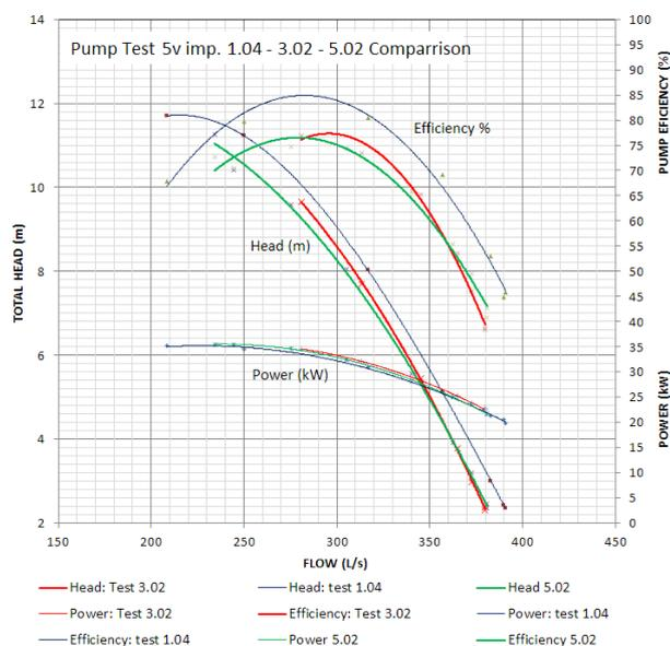
Figure 9. Pump curves for 5-vane impeller. Test numbers 1.04, 3.02 and 5.02 are explained in Table 2.
