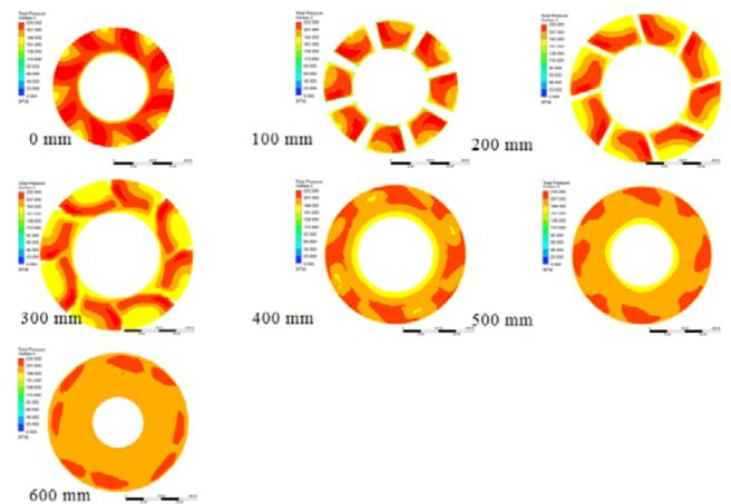
Figure 6. Total pressure on sections through the combined new-diffuser and tail-piece for eight vane impeller. Dimensions 0 mm to 600 mm indicate the distance downstream from the diffuser's inlet face.
