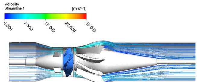
Figure 2. Five-vane-impeller 2D streamlines of new diffuser and tail-piece addition
