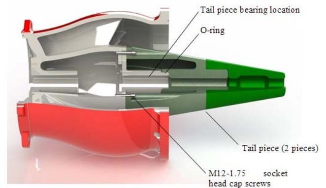
Figure 7. 3D model and installation of printed tail piece. New-diffuser (red) length is 457 mm, total tail-piece's 600 mm. Flow direction is from left to right.
