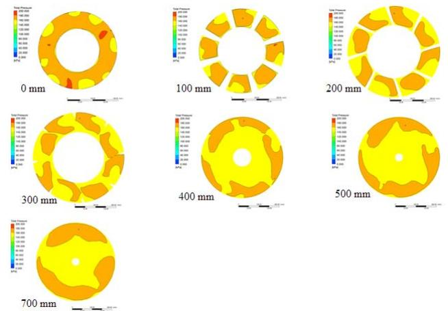
Figure 3. Total pressure on sections through the new diffuser for five vane impeller. Dimensions 0 mm to 700 mm indicate the distance downstream from the diffuser's inlet face.
