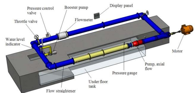
Figure 8. Pump test-rig arrangement (loop) viewed from above; flow direction counter-clockwise. Loop length 9400 mm, width 3000 mm (between pipe centre-lines); pipe's inside diameter 410 mm..
