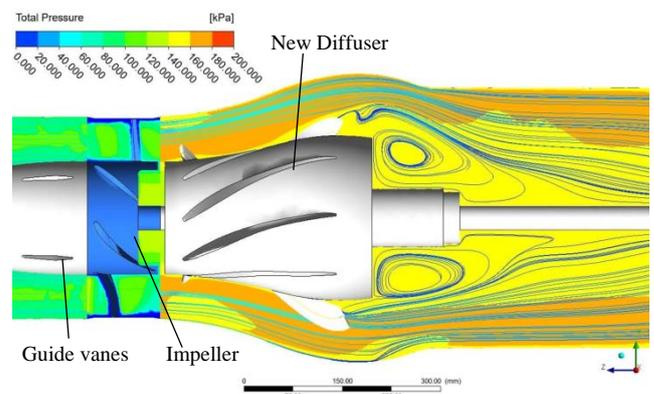
Figure 1. 2D-streamline flow-pattern and total-pressure distribution through pump with the new diffuser. Flow direction is from left to right.
