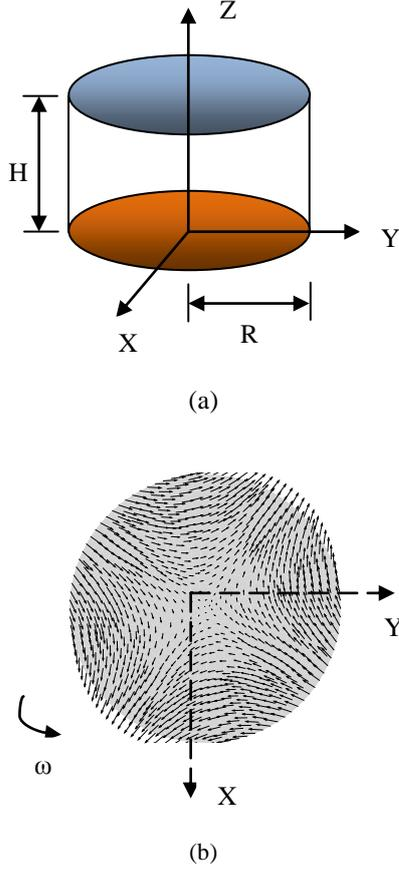
Figure 1. (a) The liquid bridge model; (b) the distribution of the magnetic lines of the non-uniform RMF on the X-Y plane.
